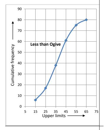
4) The following data gives the information on the observed lifetimes (in hours) of 225 electrical components. Represent in the less than ogive.
