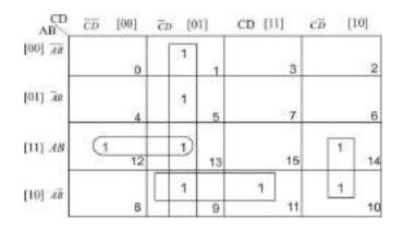
$\therefore$  Combined reduced sop expression is  $= \overline{C}D + AB\overline{C} + \overline{ABD} + AC\overline{D}$
