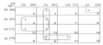
:. Combined reduced sop expression is  $F = \overline{CD} + B\overline{C} + A\overline{BD} + \overline{ABCD}$ 3. Reduce  $(A, B, C, D) = \sum (1, 5, 9, 10, 11, 12, 13, 14)$  using in K-Map.
